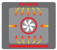
The extra-wide oven with heat-assisted convection fan and full-width broiler provides balanced air flow and even heat distribution.
