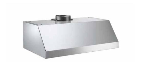
The single-motor canopy hoods deliver extraction power up to 400 CFM with three different power settings. They come equipped with aluminum mesh filters, all easily removable and dishwasher safe. They can be installed under a cabinet or on the wall with an optional narrow duct cover. The design matches Bertazzoni Professional Series ranges and cooktops while also complementing other Bertazzoni Series.
