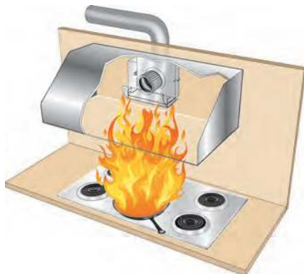
No Greasy Filter to Sustain a Secondary Fire
