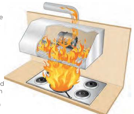
Greasy Filters and Ducting are Flammable
